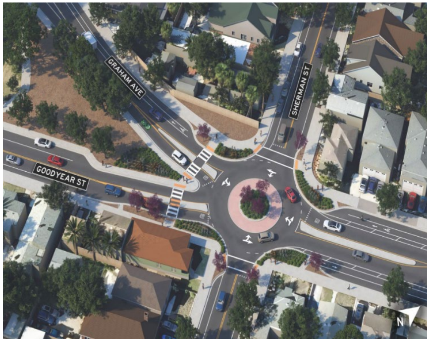
Figure 4 Conceptual roundabout design at Goodyear Street and Graham Avenue
