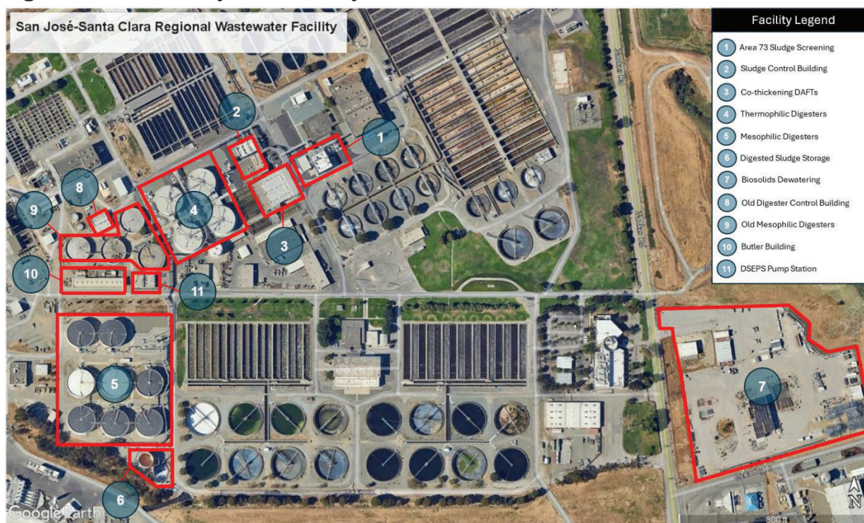
Figure 1-1 Solids System Site Layout
