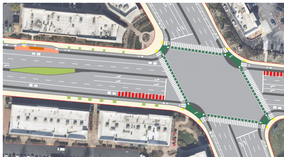
Figure 24 Planning Level Concepts for a Protected Intersection at Oakland Road and Brokaw Road
