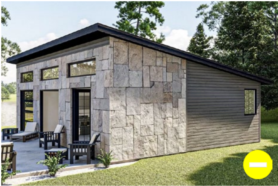
Figure 59: The size, shed roof, and detached character of this ADU are compatible with Eichler residences. However, the use of stone veneer cladding is inconsistent with the aesthetic of Eichler designs. Source: Architectural Designs.
