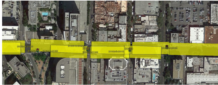
Figure 4: Geofenced zones for the radio-based EMTRAC system along Santa Clara for Rapid Route 522
