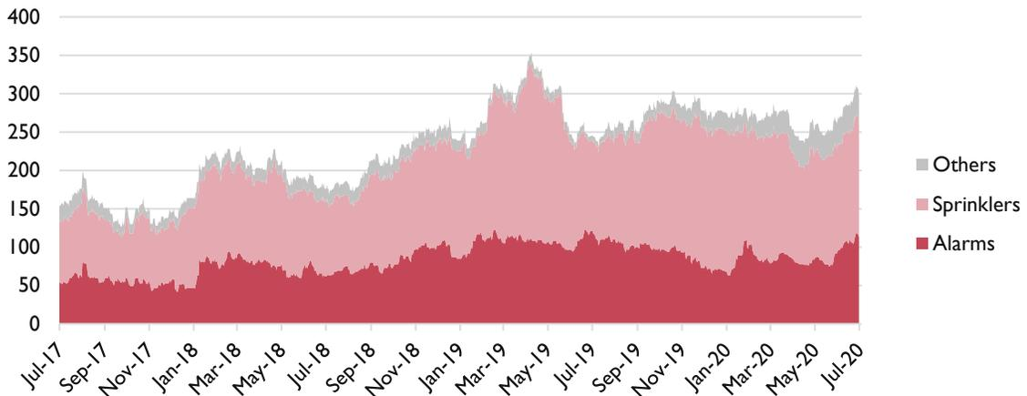
Source: Auditor analysis of AMANDA data. Graph displays the net number of plans within a discipline, based on the application intake date and the issue date (if applicable), on a given day. Does not adjust for interim review by contractors. Backlog is shown for all plans incoming as of July 2015. Other includes variances, which may be reviewed by either discipline.
