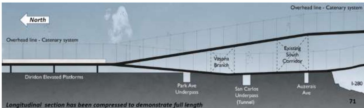
Figure 4 – Longitudinal Section of Southern Flyover
