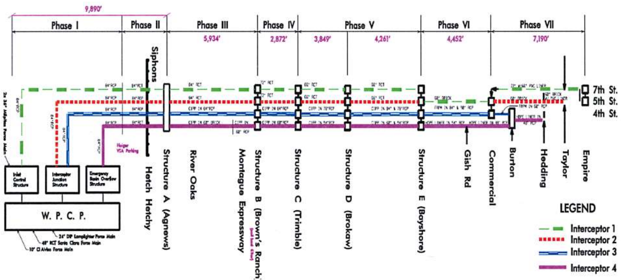
Figure 3 - Sanitary Sewer Interceptor System
