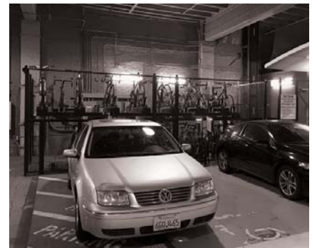
DO NOT - A separate entry for bicycles is safer than joint entry with vehicles.
