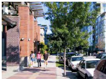
Street parking creates a buffer between pedestrians and traffic, and slows traffic down.
