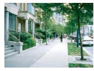
Sidewalk widths should be generous enough to accommodate a curb zone with trees, a circulation zone, and a ground floor related zone that can be used for seating, displays or bike parking.
