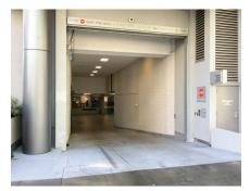
**DO** - Internal access to trash, recycling, and loading through a narrow doorway (16' in this photo) reduces impact on the sidewalk.
