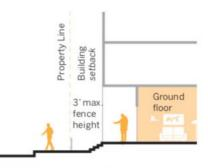
b. **DO** - Create a residential frontage with individual unit entry. Ground floor must be within 3 feet of ground level.
