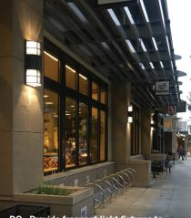
DO - Provide frequent light fixtures to create additional, more pedestrian-scale lighting than that from street lamps.
