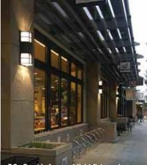
DO - Provide frequent light fixtures to create additional, more pedestrian-scale lighting than that from street lamps.
