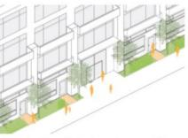
c. **DO** - An alternative to stoops for ground floor residential units is an at grade entry and internal stairs to the elevated ground floor level. Note the ground floor must still be elevated per Section 5.3.3.
