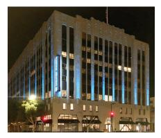
**DO** - Use *Wall Washing* to accentuate the *Podium Level*. If lights are pointed upward, avoid spilling extra light away from the building.
