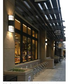
**DO** - Provide frequent light fixtures to create additional, more pedestrian-scale lighting than that from street lamps.
