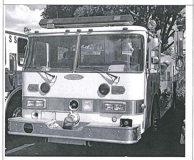
Mileage: Approximately 191,000 miles Chassis: Pierce Body: Pierce Arrow Transmission: Allison HT 740 Pump Make/Model/Capacity: Waterous,1500 GPM Water tank capacity: 500 gallons
