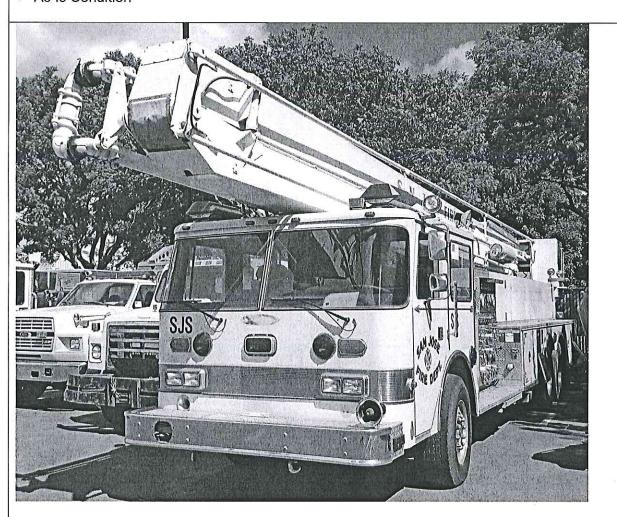
Mileage: Approximately 83,000 miles Chassis: Pierce Engine: Detroit Transmission: Allison HTB 755 Pump: Waterous, 1500 GPM
