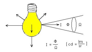
Figure 4 - Spatially Isotropic Radiation
