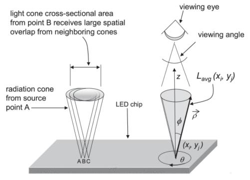
Figure 2 - Overlapping Cones<sup>2</sup>
