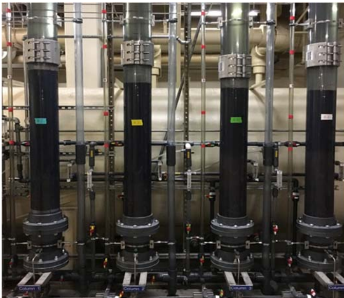
Figure 3: Four various filter media configurations tested.
