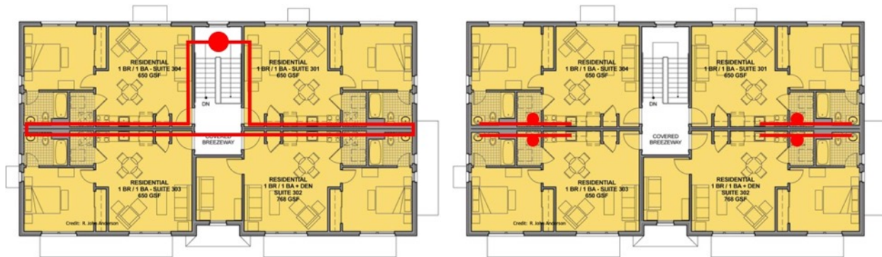
Figure 1: Central water heating with recirculation loop (left) versus individual water heaters (right) connected directly to the hot water points of use.
