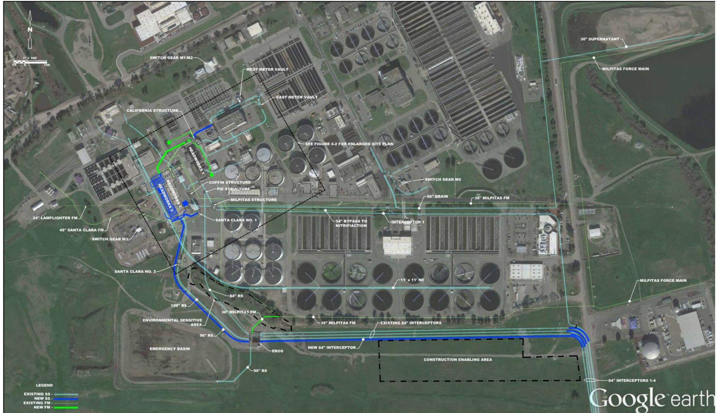
Figure 1-8 RWF Site Plan – Indicative Design of Influent Conveyance and Preliminary Treatment Improvements
