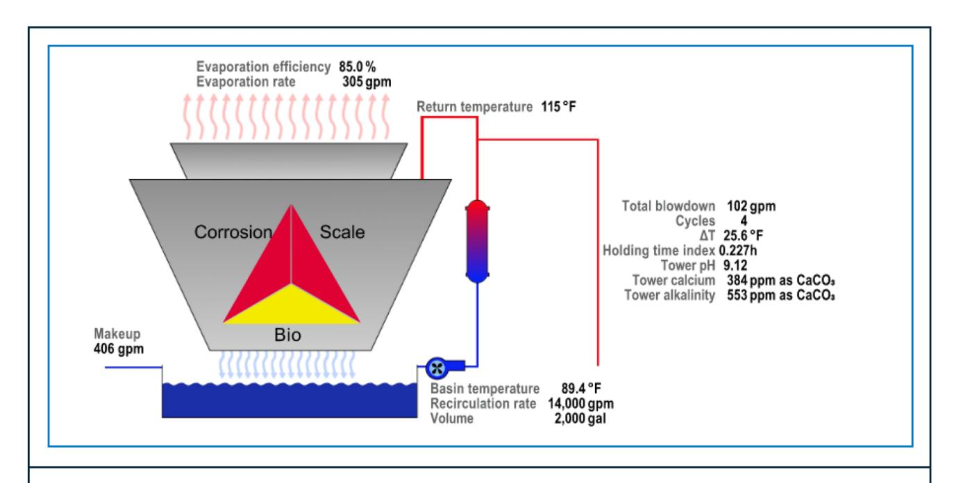
Figure 3: Cooling Tower Water Usage Diagram
