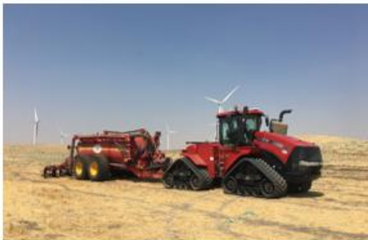
Figure 5: Subsurface Injection Equipment
