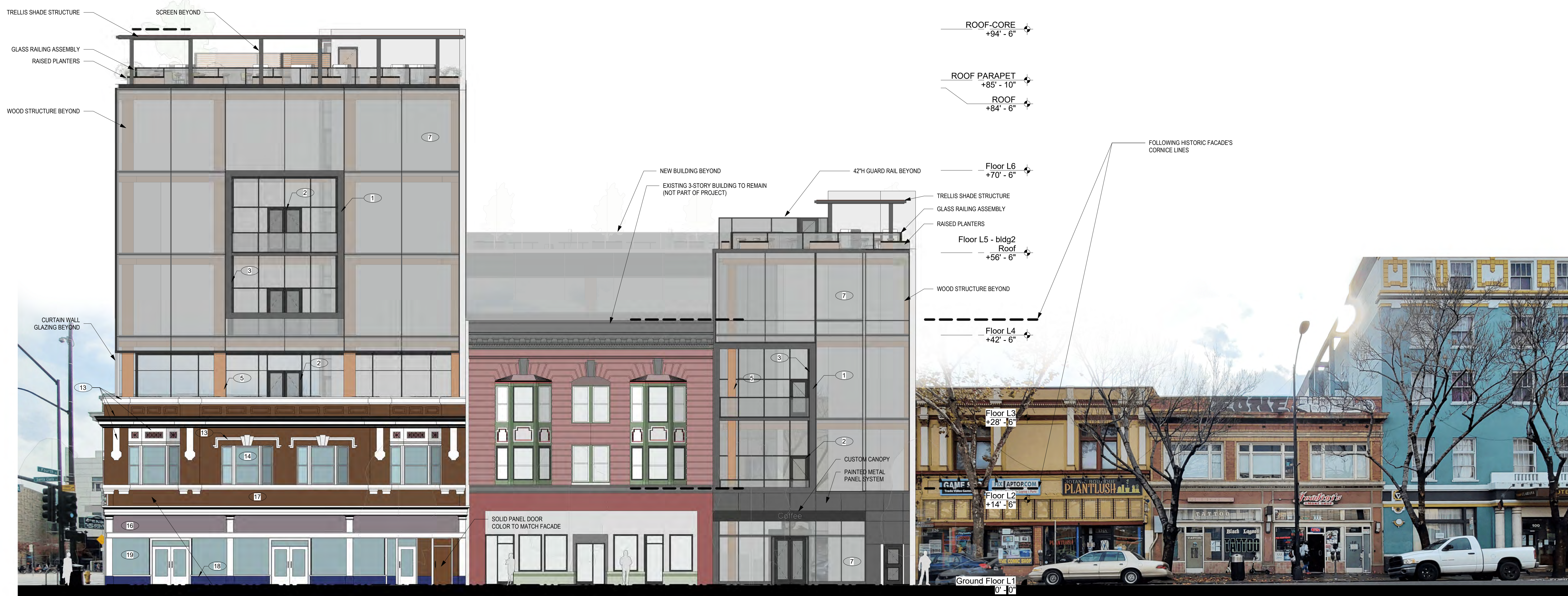
1 NORTH ELEVATION 1/8" = 1'-0" EXISTING PLASTER TO BE REMOVED ALTERNATE SOLUTION KEEP PLASTER AND REMEDIATE
