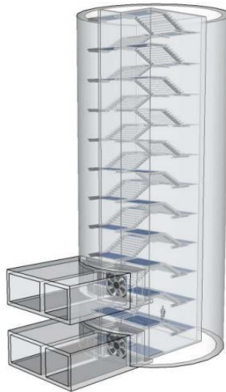
Pressurized emergency access stairs and tunnel ventilation shaft
