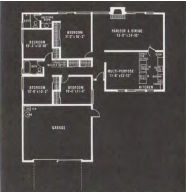
Figure 6: Example floor plan of an Eichler model with an L-shaped plan. Source: Courtesy of Sally Zarnowitz.
