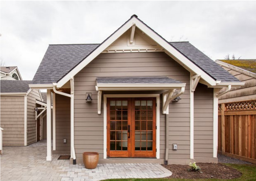
Figure 60: The size and scale of this ADU and use of horizontal wood siding are suitable for properties with Eichler residences. However, doors and windows with divided lites and decorative elements from other architectural styles, such as wood roof eave brackets, are discouraged, as they are inconsistent with Eichler designs and neighborhoods. Source: wemodallas.com.
