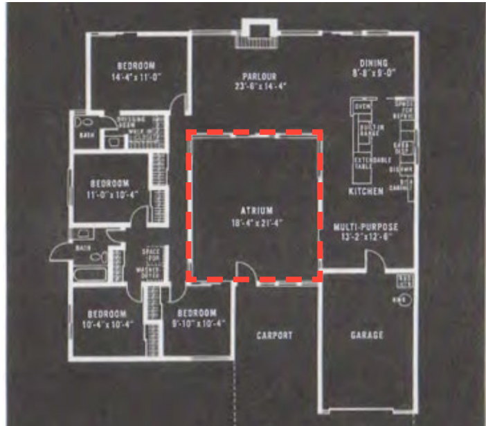
Figure 5: Example floor plan of an Eichler model with a courtyard or atrium (outlined in dashed red line). Source: Courtesy of Sally Zarnowitz. Edited by Page & Turnbull.
