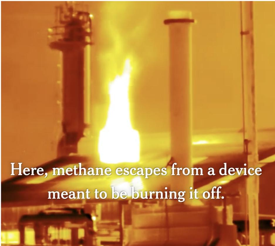
Here, methane escapes from a device meant to be burning it off.
