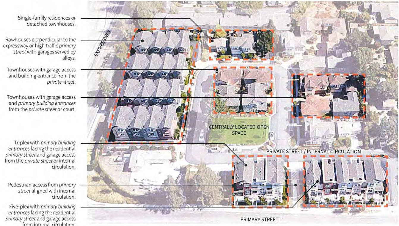
Fig. 5.11 A multi-unit development with several residential building types in a neighborhood with predominantly single-family residential developments. The site planning and organization utilizes the site efficiently and blends in with the scale and character of the rest of the neighborhood.
