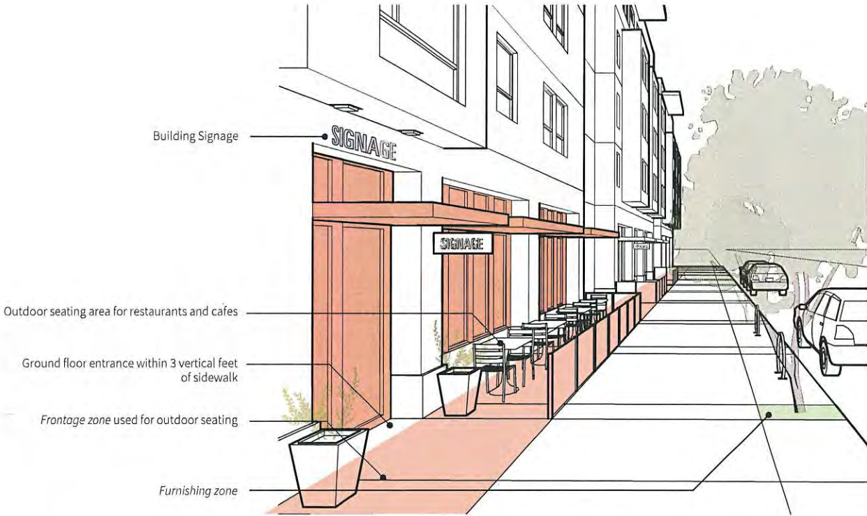
Fig. 4.4 Provide a setback for commercial frontage along primary streets to allow for transitions, frontage zones for outdoor seating, and future sidewalk widening.
