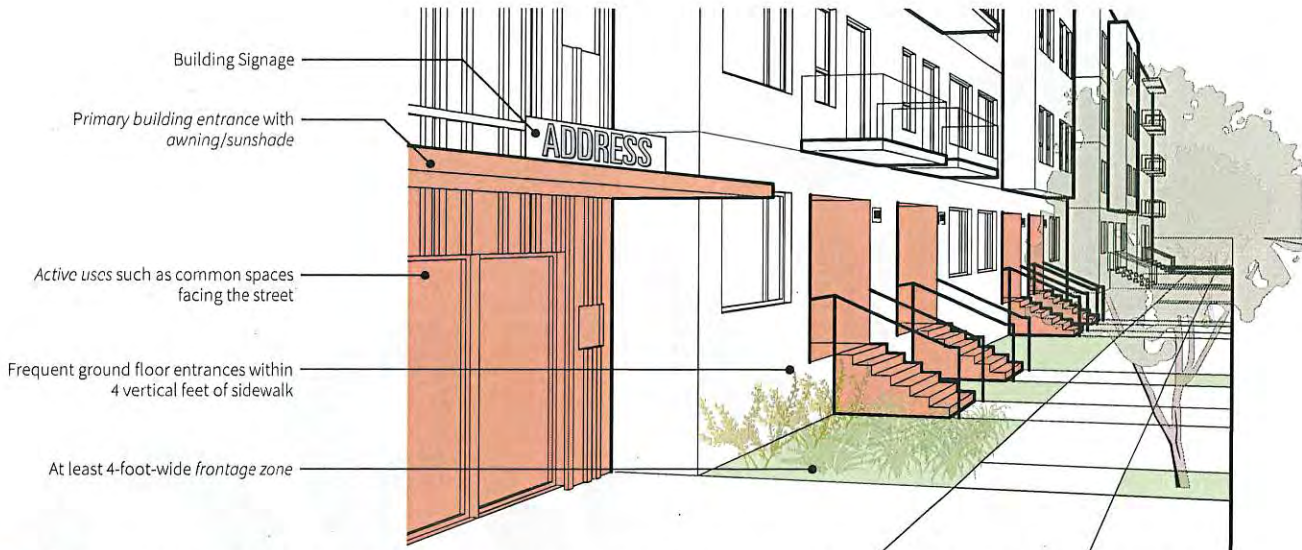
Fig. 4.8 Locate residential entrances and active uses such as gyms and community spaces on street frontages. Frontage zones create the opportunity to provide stoops for raised residential units and protect pedestrians from any doors opening out to the sidewalk.
