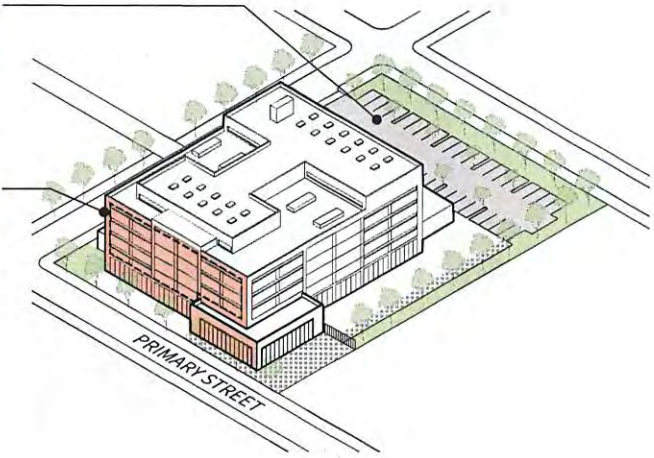
Fig. 5.42 Data center with large, flexible interior spaces that can accommodate electrical and mechanical systems. The building has façade articulations using columns, façade plane changes , and material changes.
