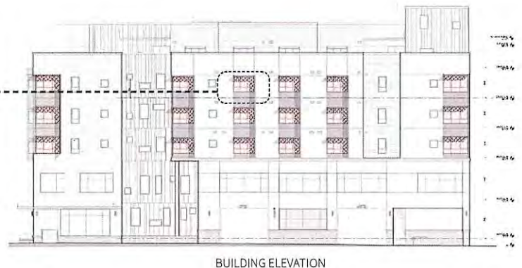
Fig. 3.37 Calculate the amount of shade on a window considering a 45° angle with the base equal to the depth of the sunshade for both horizontal and vertical shading.
