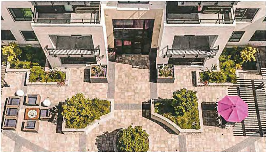
Fig. 2.39 Outdoor recreational facilities and seating designed as part of the landscape help to define on-site circulation. LID planters with native plants and permeable pavers help to mitigate stormwater and enhance the character of the development and quality of open spaces.
