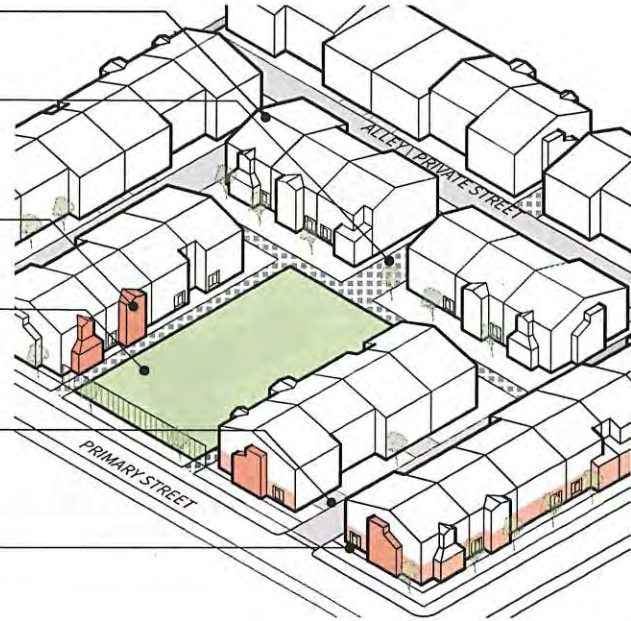
Fig. 5.6 Rowhouse Development - A rowhouse development with garages served by alleys or secondary, less prominent streets. Residential frontages have articulations that blend in with the surrounding neighborhood and provide direct access to a common open space for tenants while creating visual interest from the street.
