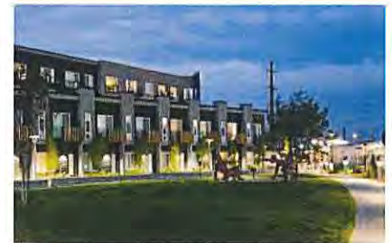
Fig. 2.35 Orient site lighting towards the building envelope or directly downwards.
