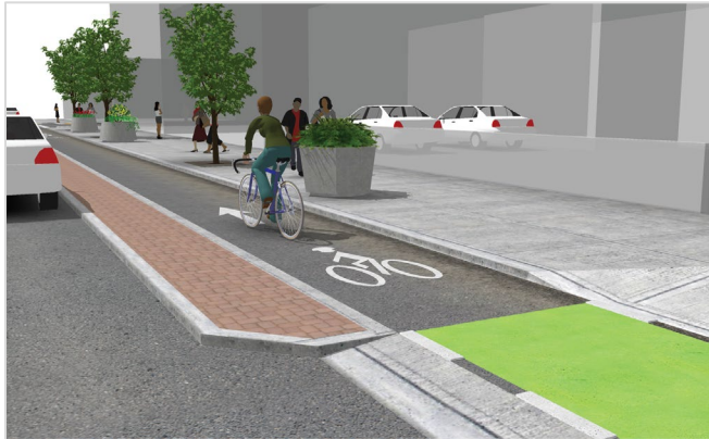
Figure 16: Raised bikeway design. (Source: NACTO)
