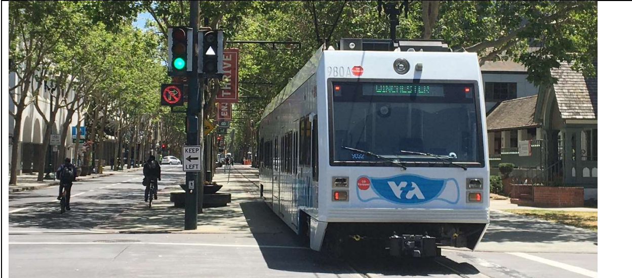
A Transit Priority Signal (White Symbol Right of Traffic Light) Gives a LRT Vehicle Permission to Enter the Intersection Before Autos, Downtown San José
