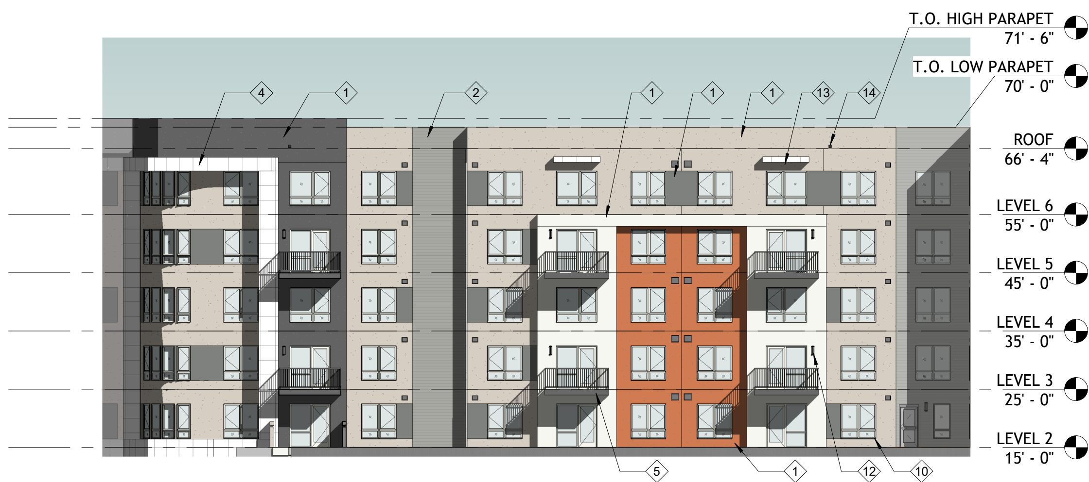
3 EAST ELEVATION - SOUTH COURTYARD 1/16" = 1'-0"
