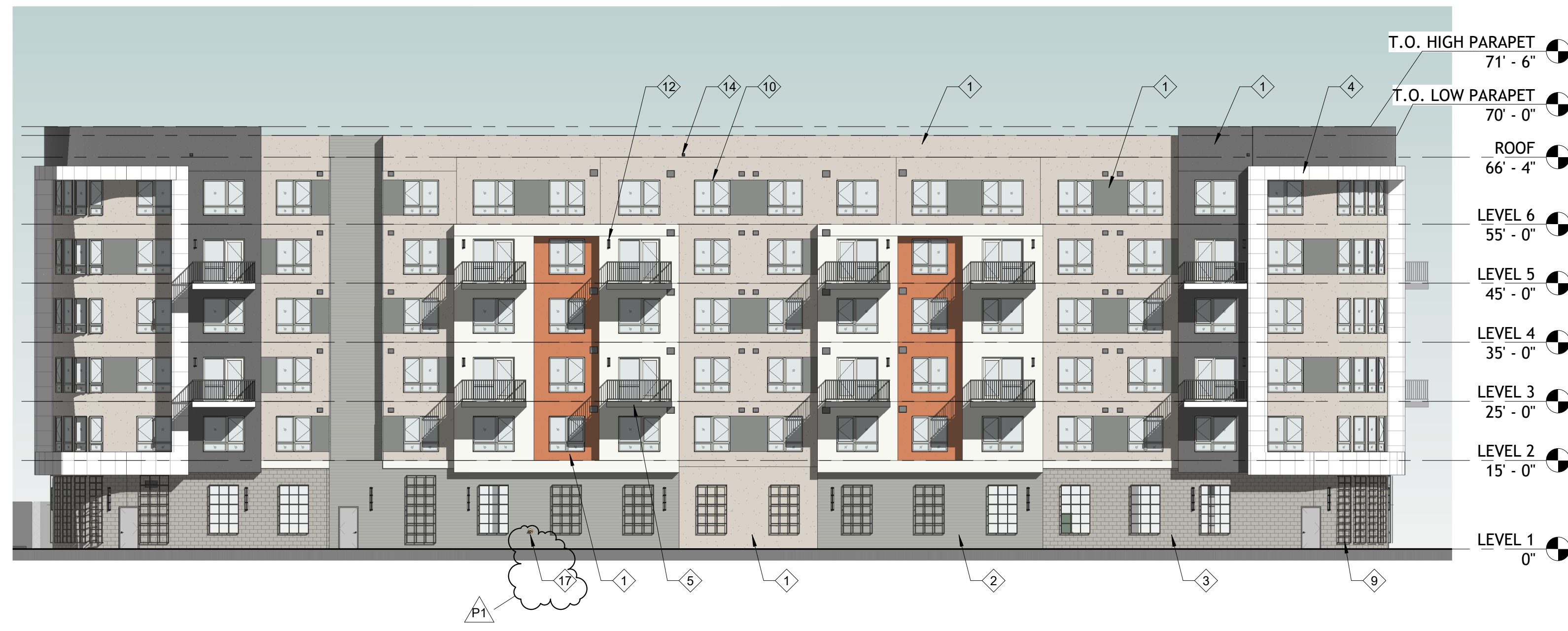
3 NORTH ELEVATION - SHORE DRIVE 1/16" = 1'-0"
