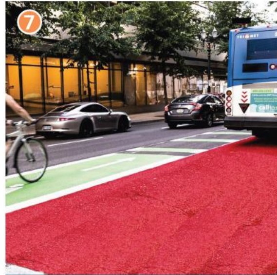
7 Dedicated lanes for buses and right-turn vehicles to improve transit speeds and reduce transit delays due to congestion
