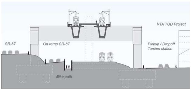
Figure 7 - Cross-section of I-280 Viaduct at Tamien Station
